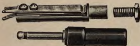
FIGS. 113 and 114.—Spring Jack and Short Answering Plug of a Sterling Metallic Circuit Switchboard. The Jack is a Brass Tube, with Springs of German Silver.
